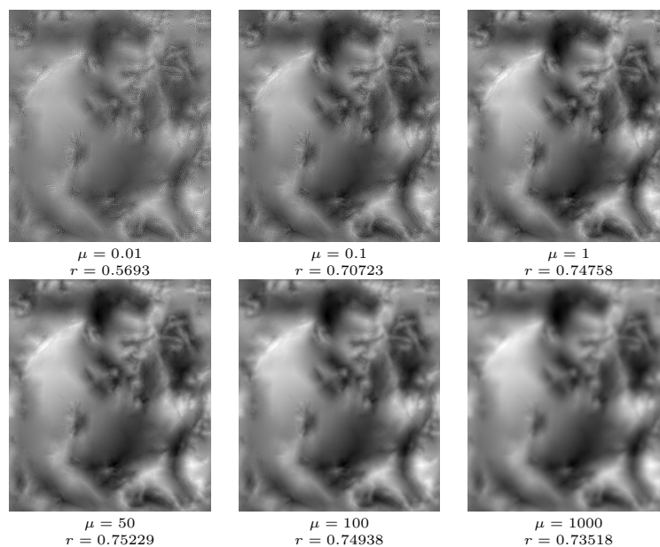
Figure 5. Influence of the regularization parameter \mu in MS-Poisson. As expected, increasing \mu penalizes more the L^2 norm of the gradient and thus makes the image blurrier. Here again we indicate the value of the normalized correlation r with respect to the original image. We empirically observed that a good compromise between recovered details and smoothness is often attained around \mu = 50 . (Images are better seen in the electronic version.)
