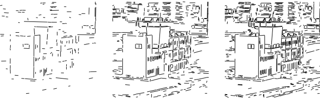
Fig. 12 Output of the LSD algorithm on respectively, from left to right : the image reconstructed from the sample of P_0 and R_{100} , the image reconstructed from the sample of Q_0 and R_{100} (these two images are the ones of the last row of Figure 9), and the original Pirée image I^0 . Notice how the last two images are very similar.
