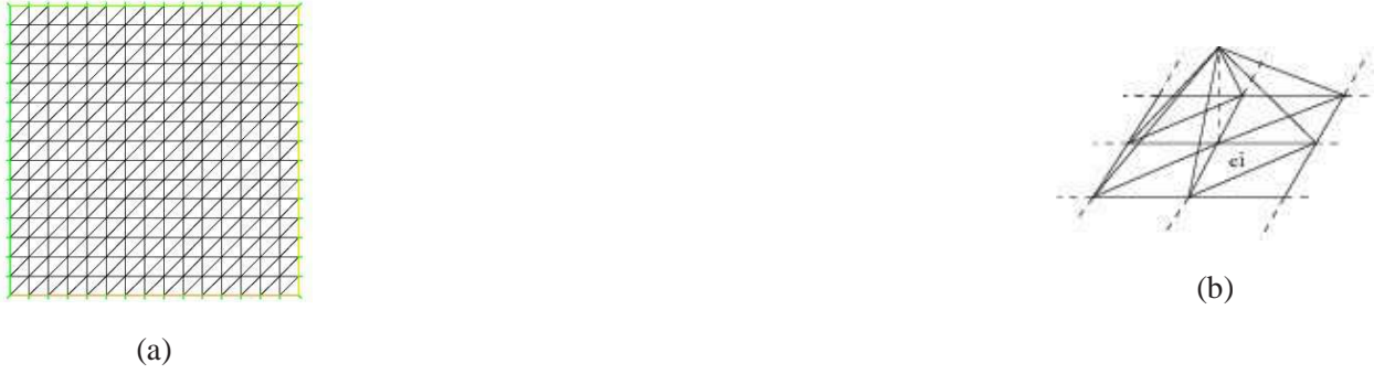
Fig. 1. Discretization of the deformations domain \Omega : (a) The mesh, (b) a P1 -Lagrange finite element function \Phi_i is associated to a vertex e_i (piecewise affine function).
